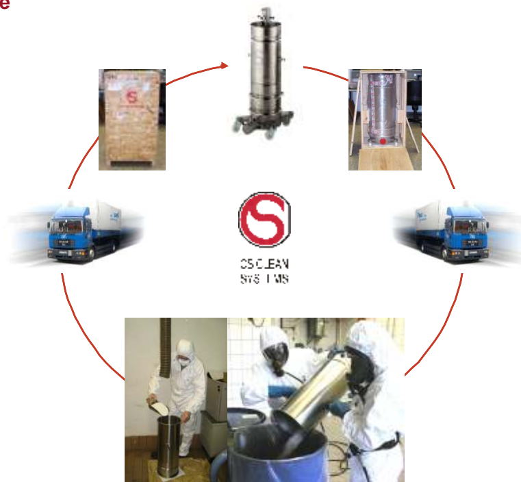
Refill cycle of spent absorber columns
